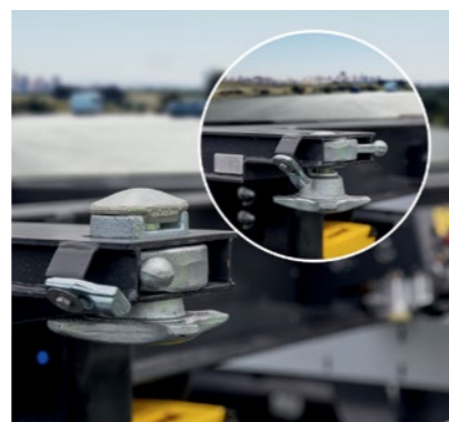
Galvanised container lock with anti-twist device, retractable for driving underneath swap bodies
