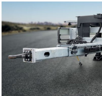
Telescopic draw tube* (4x100 mm) with mechanical locking (Z.WF)
