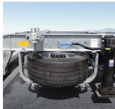
Spare wheel holder in basket design and two-sided support winch on rear frame, with one-sided operation on the right, balancing foot and two gear steps (Z.WF)
