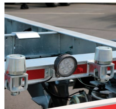
Two pairs of galvanised guide rollers (optionally three pairs: front, centre and rear) as well as additional working lights* (LED version) on the front and rear container support beams
