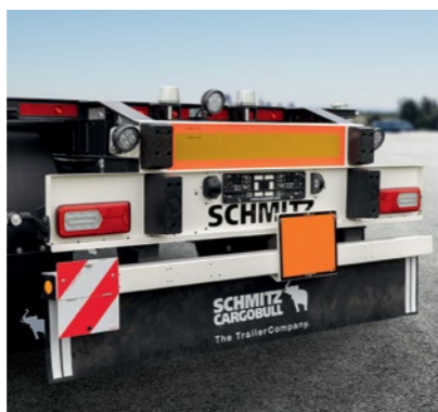
Bevelled upper flange on the chassis at the rear of the A.WF, suitable for better reception of swap bodies
