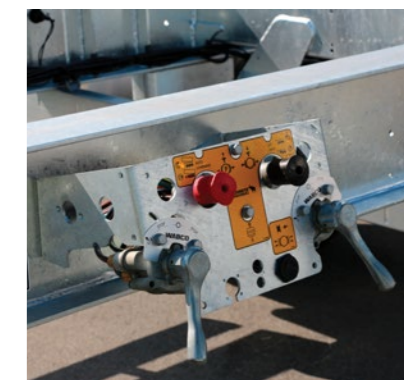
Control unit for parking brake and airsuspension with two lifting and lowering valves on the side of the solebar of the A.WF (one lifting and lowering valve on the Z.WF)
