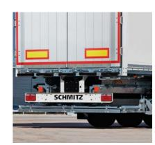
Under-ride tail lift\* for distribution transport, loading and unloading without ramp.
