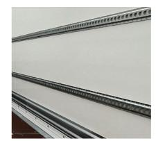
Attached load securing rails\* for horizontal beams, tension belts and securing tarpaulin.
