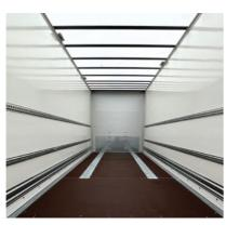
Aluminum end wall with galvanized steel base scuff plate: protection for cargoand trailer
