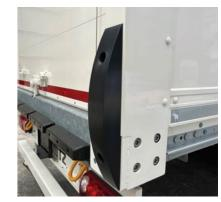
Heavy duty corner protection\* in combination with roller shutter\* for fast access at the ramp and in distribution traffic
