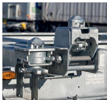
With 2 x 20' loads, the height-adjustable KLAPP LOCK takes over the locking of the front container.
