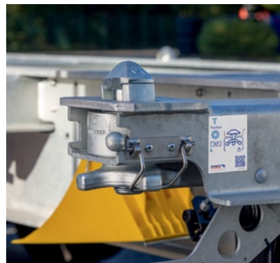
Twist locks with protection against twisting on four pairs of container beams as standard locking system.
