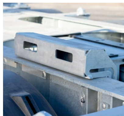
Three pairs of folding container supports* for containers without a tunnel.
