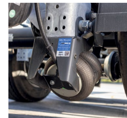
The lift axle* as a starting aid extends the wheelbase and increases the pressure on the drive axle. Unloaded, the lifted position reduces tyre wear.
