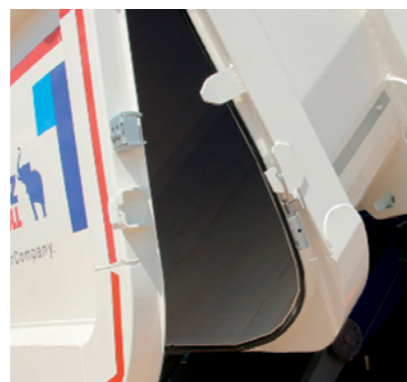
Surface-mounted rear wall flap with circumferential rubber seal.
