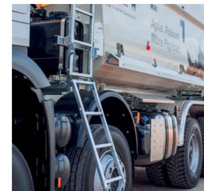
Extensive additional equipment optionally selectable: e.g. side access ladder for load control.
