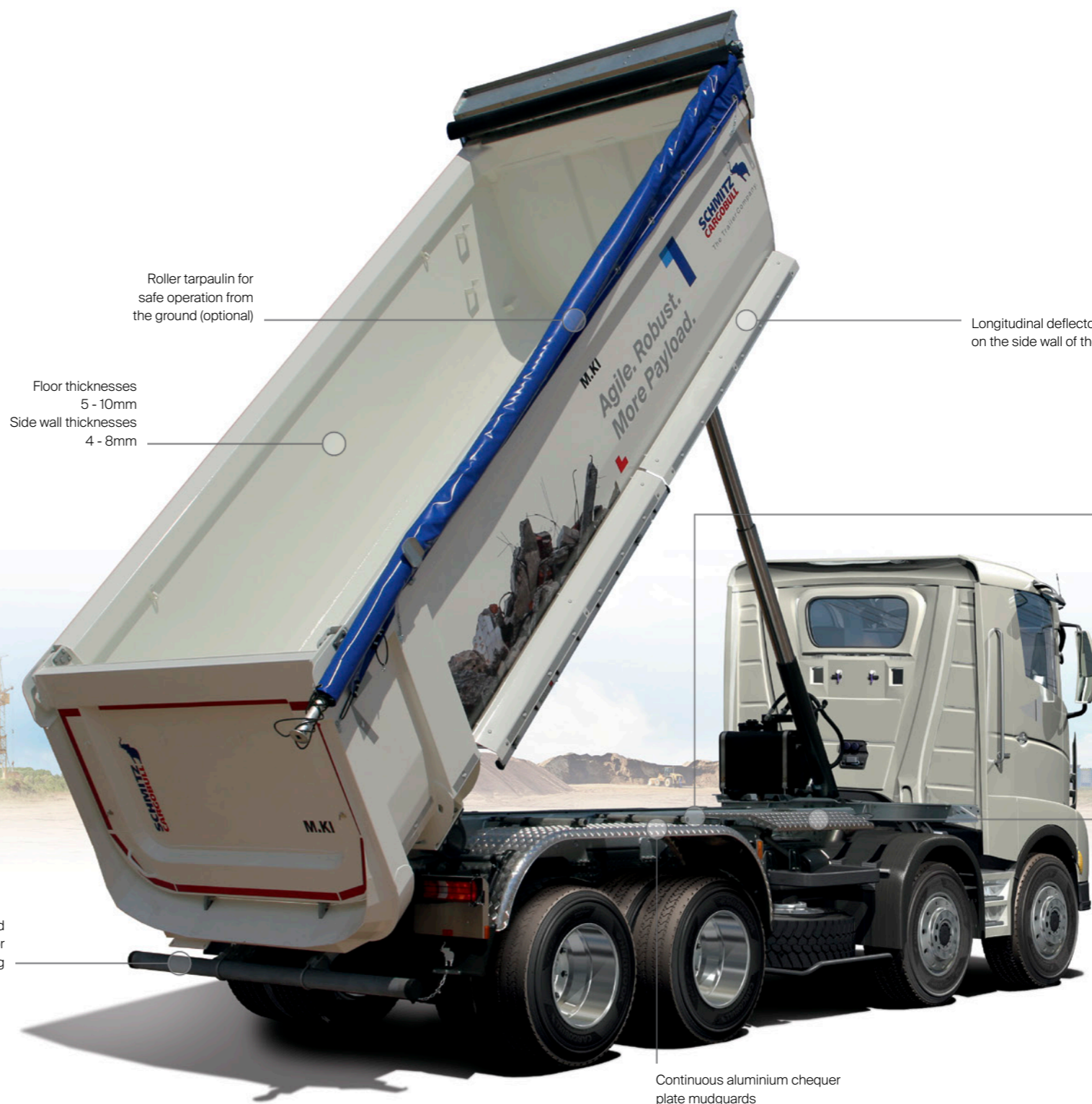
Foldable underride guard Optional: cranked version for vehicles with trailer coupling
