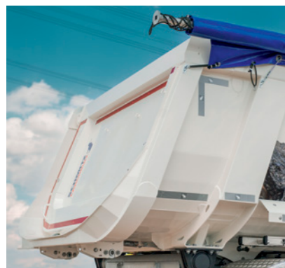
Interior pendulum flap with chute.
